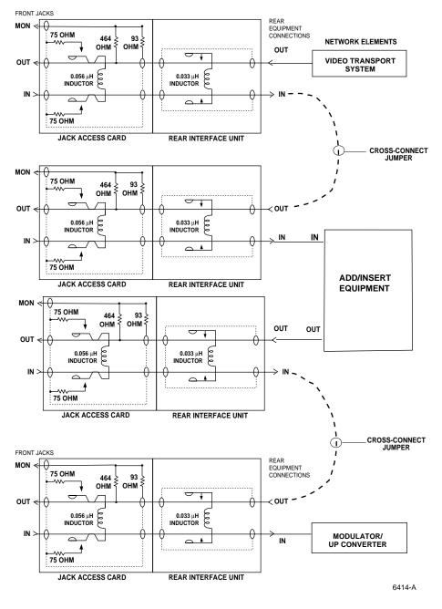
Figure 18. Cross-Connect Application for Local Commercial Insertion
